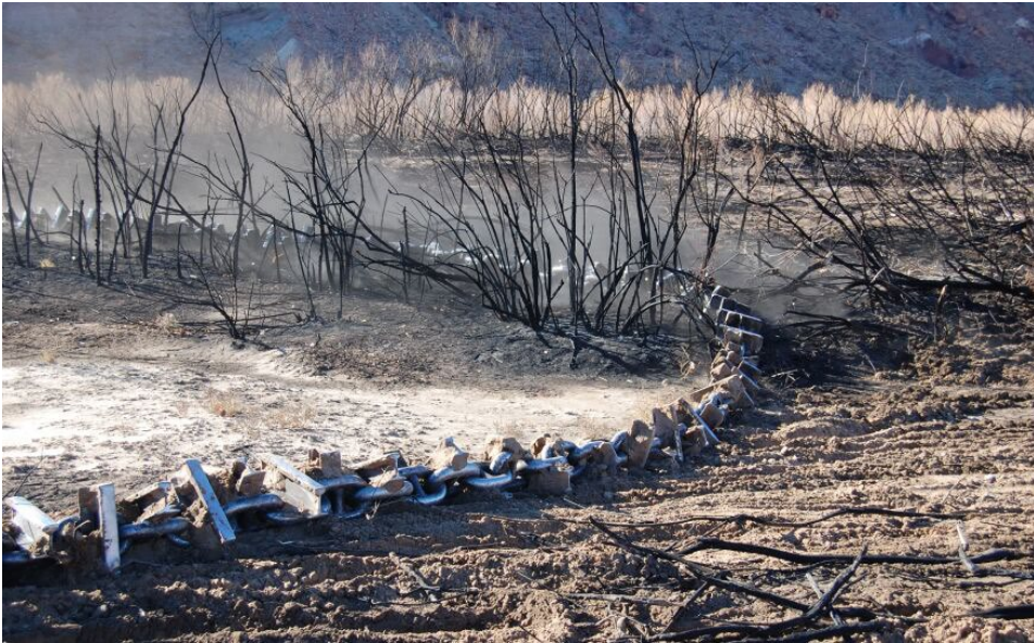
Figure 28. Chaining can be used on rugged terrain to knock down shrubs and small trees
