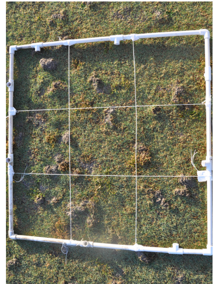
Figure 13. Testing for damage ratings is performed on 1 x 1 meter squares of soil.
