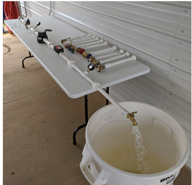
Figure 2. The flow test fixture consisted of a flow control valve, pressure regulator, pressure gauge, calibrated water meter, digital flow meter, pressure gauge, and test valve. Each of the five valve types were connected to the union at the end of the table for testing. Shown is testing open pipe flow with no valve (left) and hose bibb 1 (right) with the same water supply.
