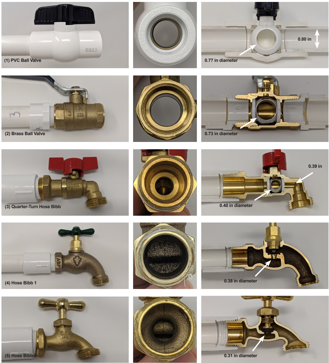
Figure 3. Side profile (left), valve entrance view (center), and internal cutaway of each valve tested.
