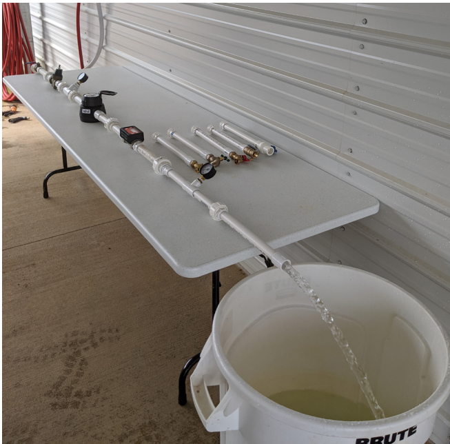
Figure 2. The flow test fixture consisted of a flow control valve, pressure regulator, pressure gauge, calibrated water meter, digital flow meter, pressure gauge, and test valve. Each of the five valve types were connected to the union at the end of the table for testing. Shown is testing open pipe flow with no valve (left) and hose bibb 1 (right) with the same water supply.
