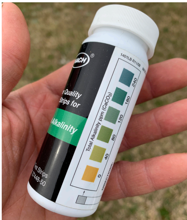
Figure 1. Simple pool test kits generally do not provide a fine enough scale to test pond water accurately.
